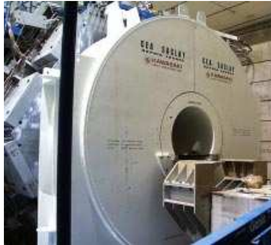
(b) Upper, or moveable, part of inner cylinder in machining
