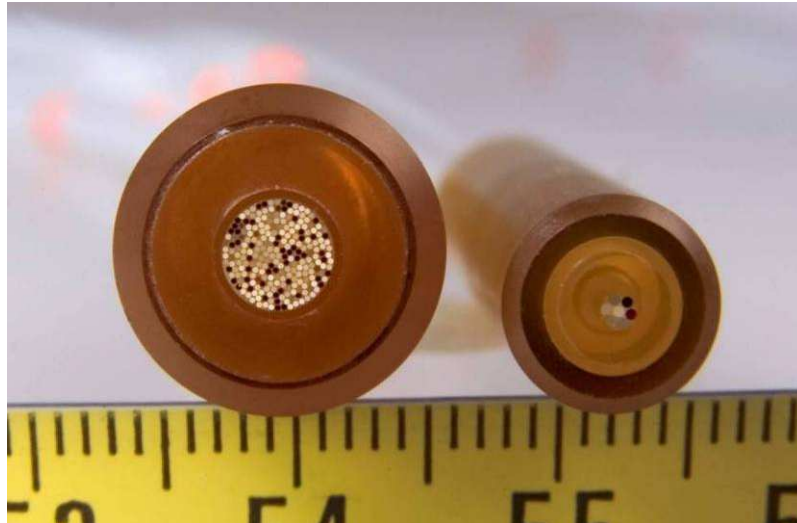
Figure 12. Polished fiber-bundle tube faces (fibers are bonded into the insert, outer ring is bundle tube): at left, 240-fiber barrel Tertiary (L1) fan-out and at right, 7-fiber Secondary (L2) fan-out. Dark fibers in the photo have color-coded protection caps to indicate that they have been selected or rejected.
