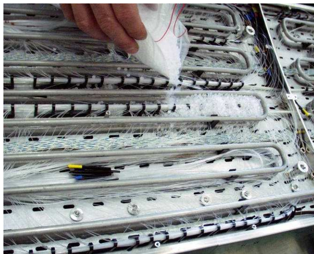
Figure 17. Molded polyethylene grains, used as a neutron moderator, are filled into the region occupied by the monitoring system before the front cover of the SM is mounted.
