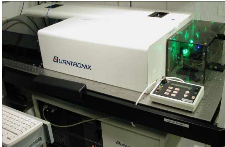
Figure 3. The monitoring system multiple wavelength light source (shown installed at CERN H4 test beam area).
