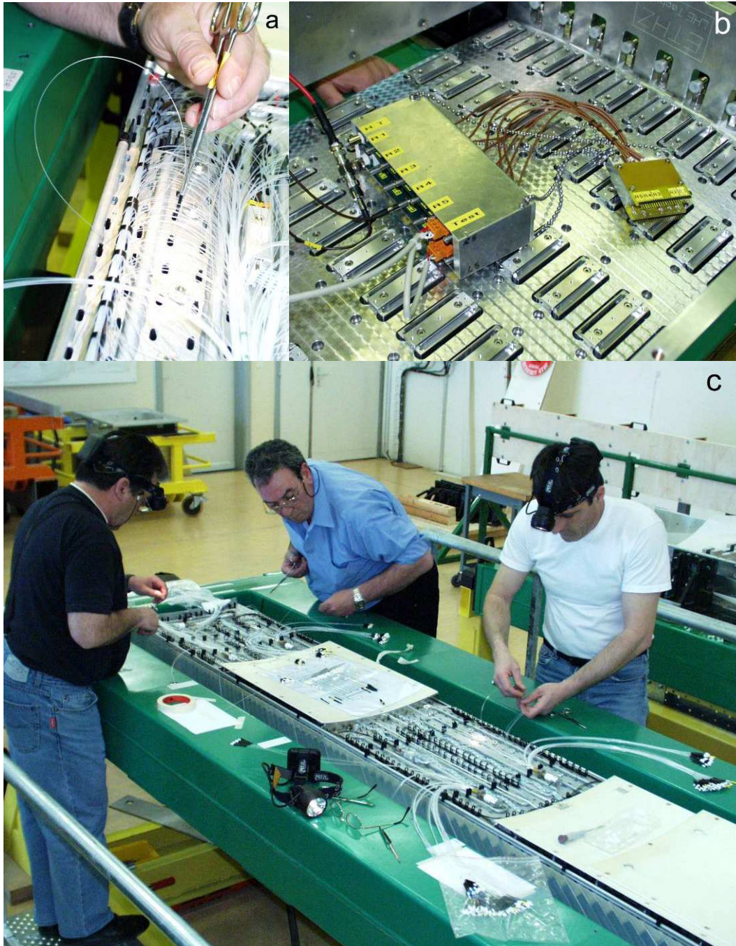
Figure 29. Installation of the monitoring distribution system on an ECAL barrel SM: (a) shows tool used to insert the optical fiber's ferrule into a crystal's ferrule support, (b) shows the 10-channel amplifier and connector used to test APD response after cabling (SM face down), and (c) shows the installation of optical fibers on alternate sub-modules (SM rotated front-face up).
