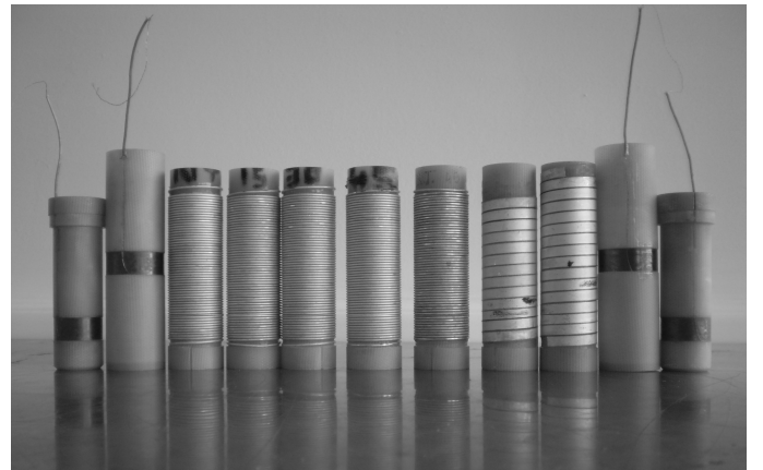
Fig. 3. The “speedy” test samples. On the left the Bi2212 ribbons after transfer on the measurement mandrels. On the right the outer and inner pick up winding used to measure the losses.
