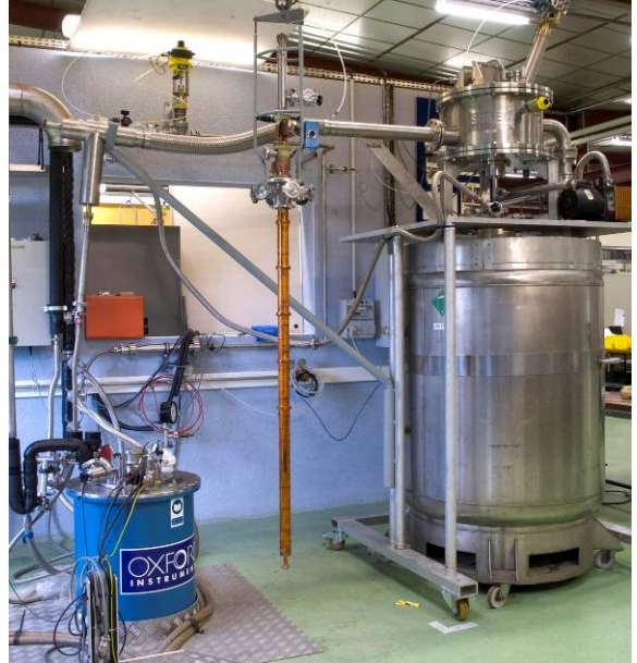
Fig. 2. The CETACE test station: on the right the helium tank with the gas exchanger on its top, in the middle the cryogenic insert, on the left the superconducting magnet.
