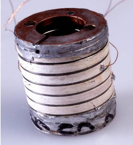
Fig. 1. Bi2212 ribbon on an adapted vamas mandrel.
