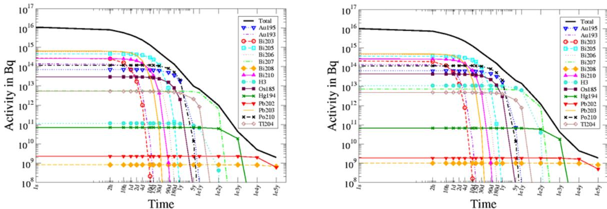
**Figure 5:** Main contributors to the activity of the LBE, as a function of cooling time after 123 days of irradiation with 575 MeV protons at 0.947 mA using INCL4-ABLA (left panel) and Bertini-Dresner (right panel) models.
