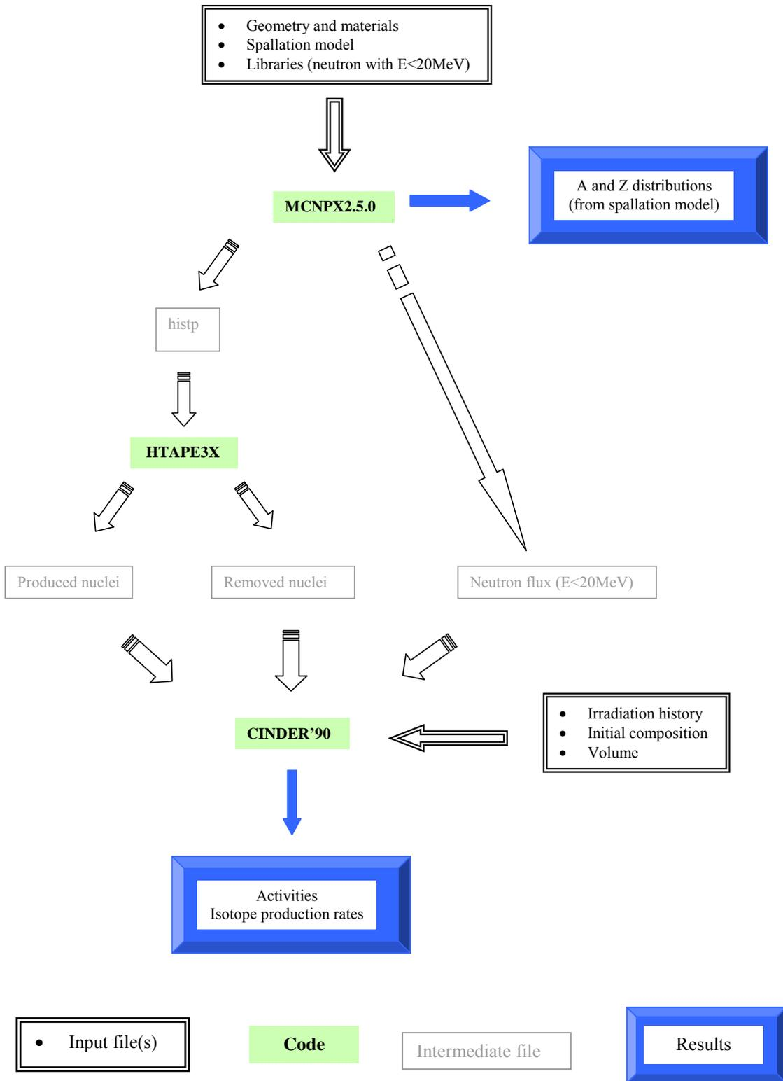
**Figure 2:** Schematic view of the calculation methodology
