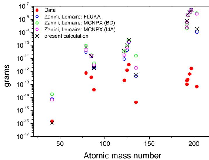
**Figure 12:** Comparison of different calculations with measurements of volatile elements released in the expansion volume of the LBE among which INCL4-ABLA and Bertini-Dresner denoted respectively MCNPX (I4A) and MCNPX (BD) in the legend.
