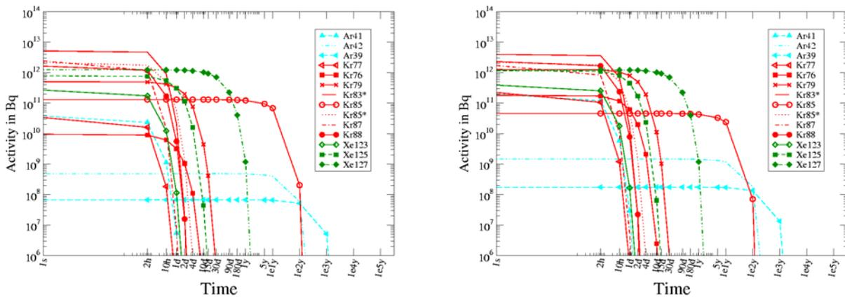
**Figure 11:** Main contributors to the activity in LBE coming from gaseous elements as a function of cooling time using INCL4-ABLA (left) and Bertini-Dresner (right).
