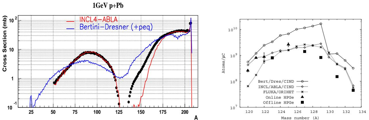
**Figure 9:** Left: Comparison of INCL4-ABLA and Bertini-Dresner predictions with the production cross-sections as a function of the residue masses measured at GSI for the p+Pb system [16]. Right: Production rates of Xe isotopes from a thick Pb-Bi target, bombarded with 1.4 GeV protons, measured at ISOLDE, compared to different calculation. From [18].
