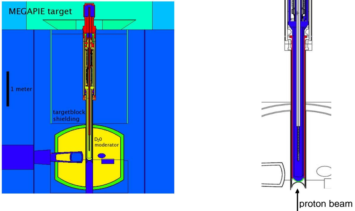
**Figure 1:** MCNPX 2D visualization of the simulated system. Left: the whole SINQ facility. Right: the lower part of the MEGAPIE target. The LBE is colored in blue, the container in red and green and its bottom part, the window, in green. Figures are drawn from [10]
