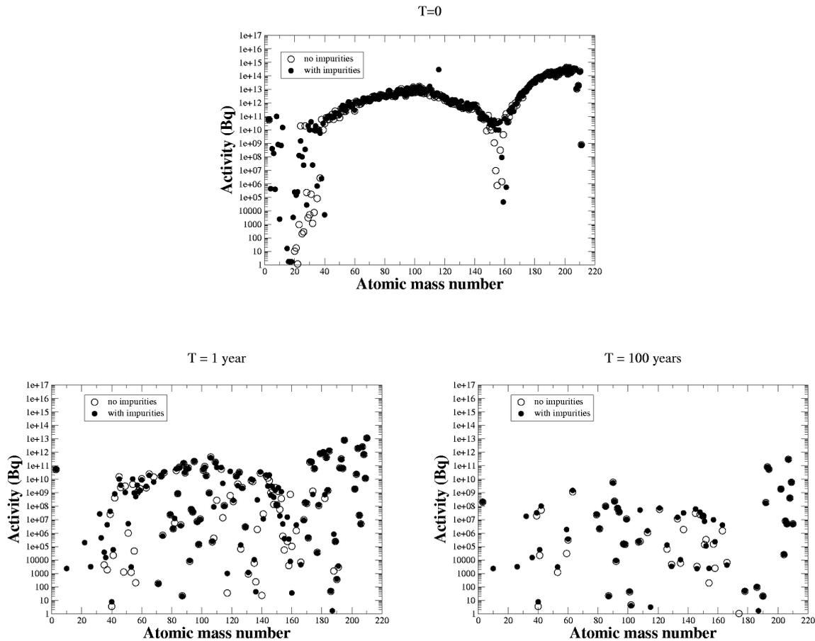
**Figure 14:** The activity of the different radionuclides, with (empty circles) and without (filled circles) impurities, as a function of their mass number, contained in the LBE after 123 days of irradiation with 575 MeV protons at 0.947 mA: just at the end of irradiation (top), after 1 year (bottom left) and 100 years (bottom right) of cooling time. The calculations are done with INCL4-ABLA.
