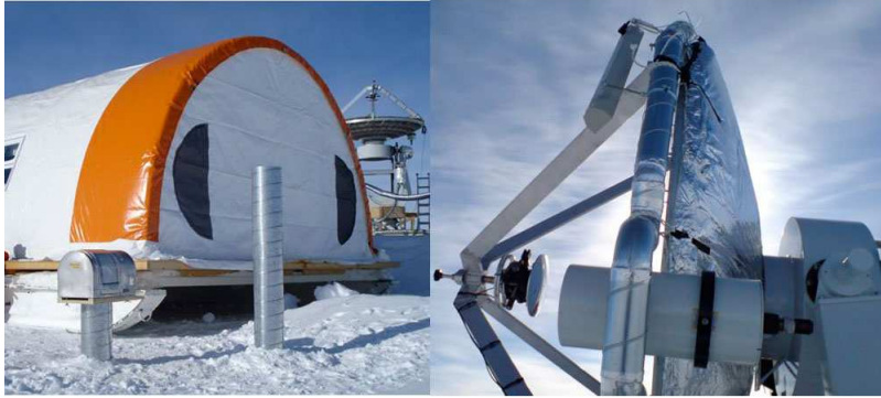
Fig. 13. Left: A submm tipper experiment to measure the transmission at 200 \mu\text{m} . Right: GIVRE on Cochise: The process of ice formation and the way of protecting the instruments are described. A 2.6-m telescope (COCHISE) will be defrosted using several methods. GIVRE will also measure other parameters that are common prerequisites for the design of unmanned telescopes at altitudes up to 45 m including the ongoing measurements of wind, humidity, and temperature.
