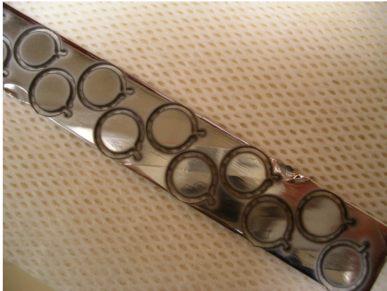
Figure 6: FG samples ( \varnothing 8 mm) cut by water-jet; Nb sheet (140 x 10 mm) was electropolished first.
