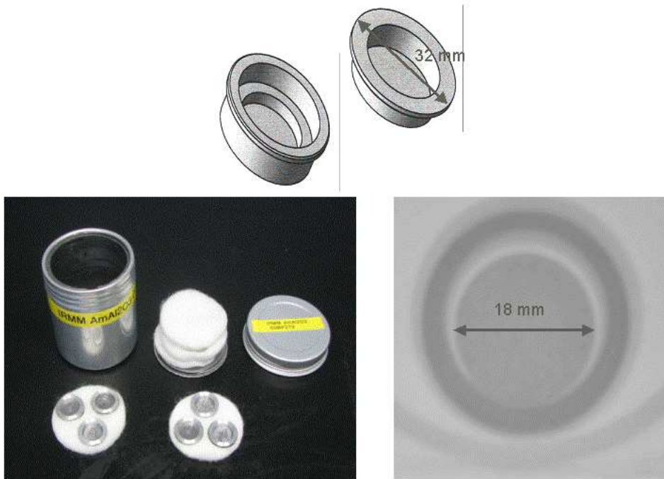
Figure 3.2: Americium samples and sample holders picture, scheme and X-ray radiograph.
