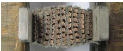
Fig. 8. SII cross-section after compression till 30 MPa.
