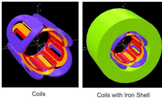
Figure 3. Superconducting multipole [Argonne National Lab.]
