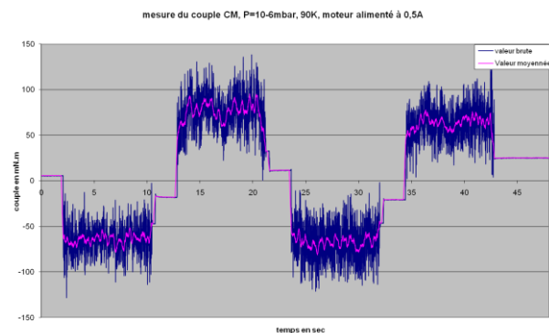
Figure 9: torque measurement (mN.m) vs time (sec). This graph plots gross results, CM friction torque is calculated from these data.
