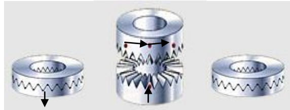
Figure 2: dog clutch operation principle
