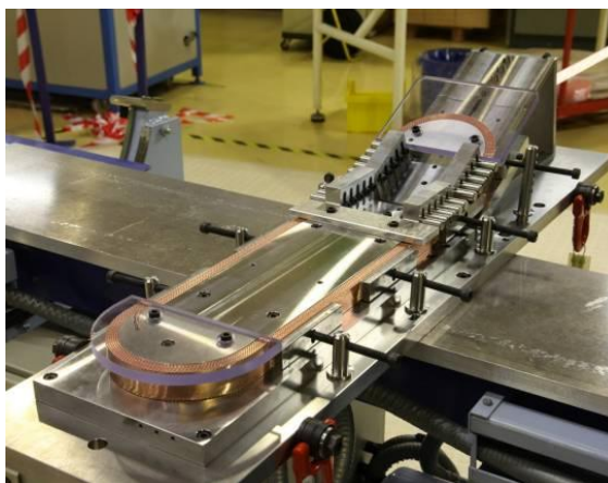
Fig. 5.2.2. Bending test tooling (final configuration)
