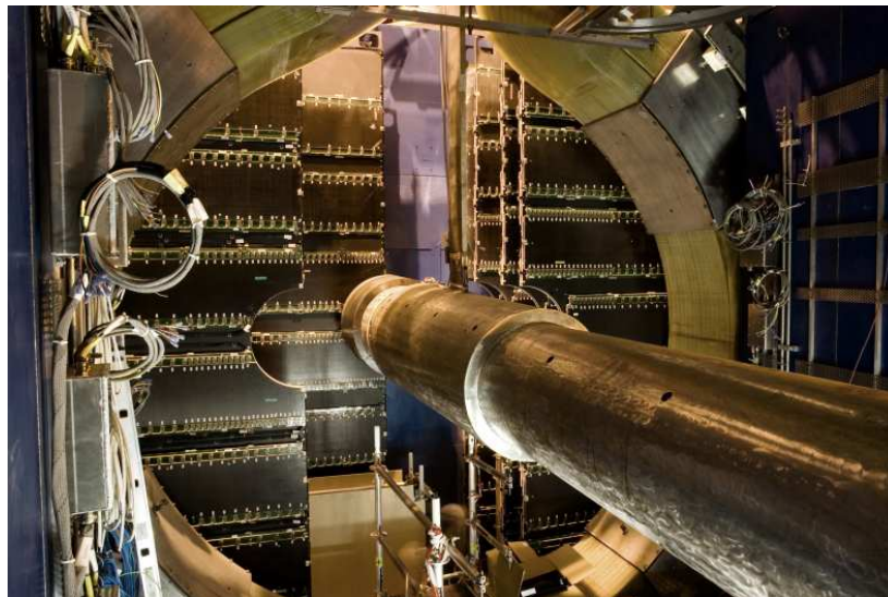
(b) Layout of stations 4 and 5 (slat architecture) of the tracking system. Read-out electronics is implemented on the top and bottom part of the slat.
