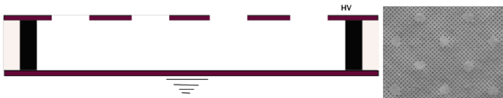
Figure 2. Left: Kapton pillars are created with a step of about 500 microns; Right: photo of a mesh with copper spots used to protect the polyimide bellow during etching in order to form the pillars.
