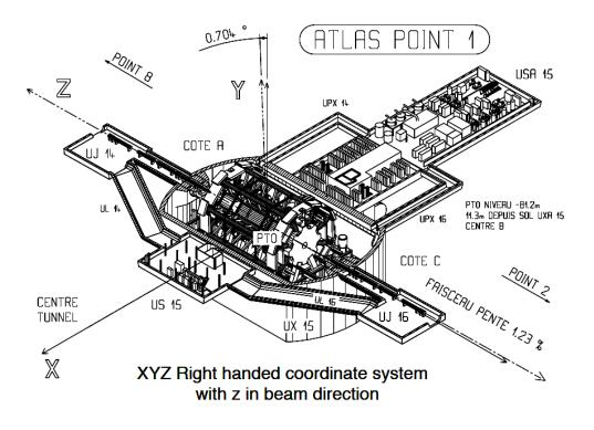
Figure 2.7: The coordinate system of the ATLAS detector.
