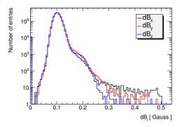
Figure 3.3: Distributions of  $dB_x$ ,  $dB_y$  and  $dB_z$  (G) measuremets taken by all sensors during 2011.
