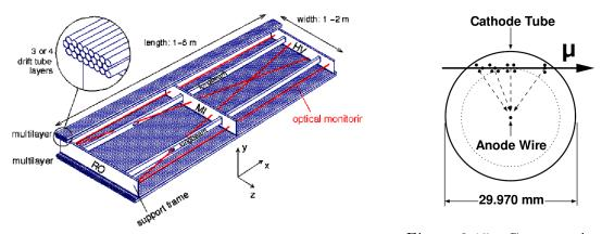
Figure 2.14: A detailed view of a muon chamber.
