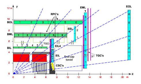
Figure 2.13: Cross-sectional view of ATLAS in the r-z projection at  $\phi \approx \pi/2$ . The Barrel MDT chambers are shown in green, the End Cap MDT chambers are blue. In the Barrel (End Caps), the RPC (TGC) chambers are shown outlined in black (solid purple)
