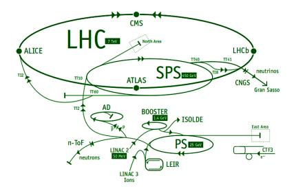
Figure 2.1: The CERN accelerator complex.
