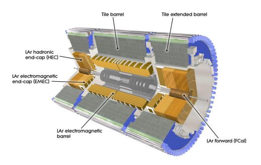
Figure 2.10: The ATLAS calorimeters.
