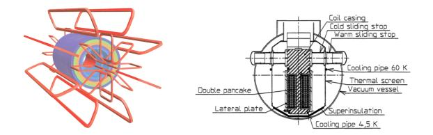
Figure 2.19: The coils of the Barrel and End Cap Toroids.
