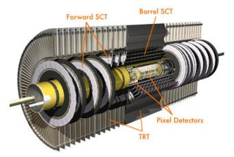
Figure 2.9: Cut away view of the Inner Detector.
