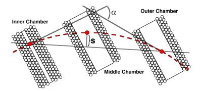
Figure 2.17: Sagitta illustration of a muon hitting the three MS layers.
