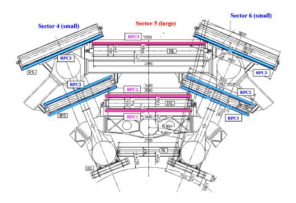
Figure 2.16: RPCs location on the middle and outer Barrel layers.
