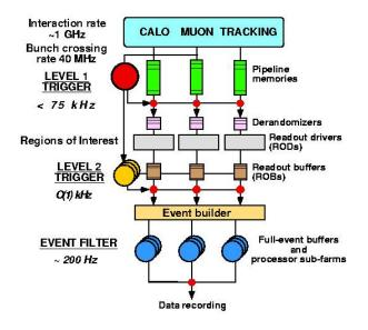
Figure 2.8: Schema of the ATLAS trigger system.
