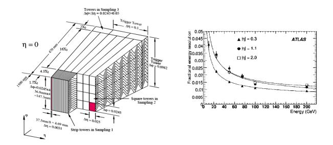
Figure 2.11: The structure of the barrel accordion calorimeter.
