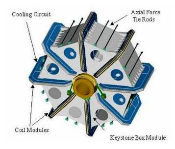
Figure 2.22: The End Cap Toroid cold mass.
