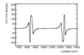
Figure 3.31: Magnetic field gradient G/1mm vs z position for x=2000mm and y=2000mm .
