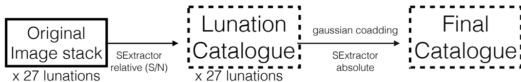
FIGURE 5.4 Detection of transient events as in SNLS3 for each virtual CCD. Boxes with continuous lines represent an image ( fits ) and boxes with dashed lines represent catalogues ( ascii ).
