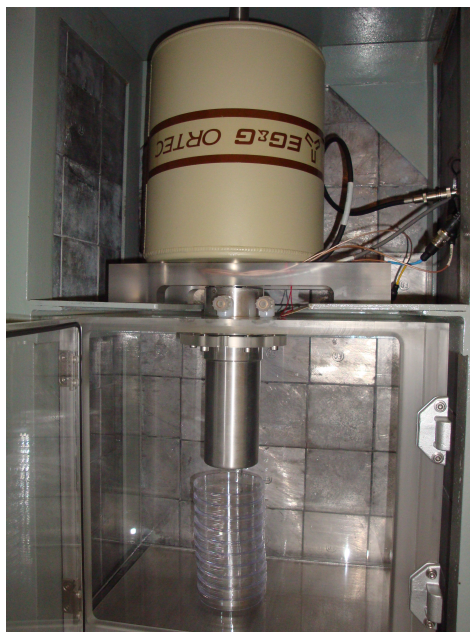
Figure B.1: Picture of the germanium counter in its airtight acrylic box.
