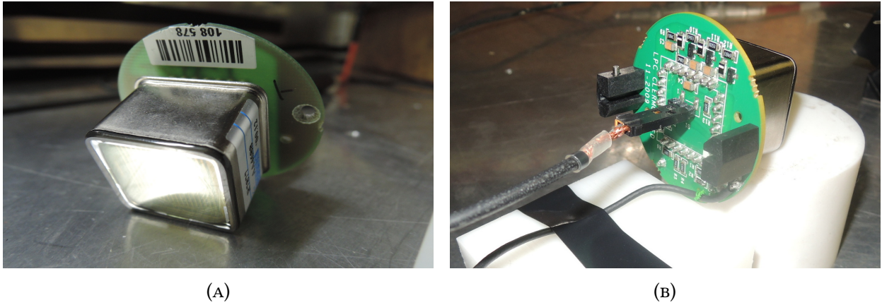
FIGURE 9.4: A Hamamatsu R7877 PMT mounted to a TileCal VD (A). The PMT signal is extracted directly from the VD (B).
