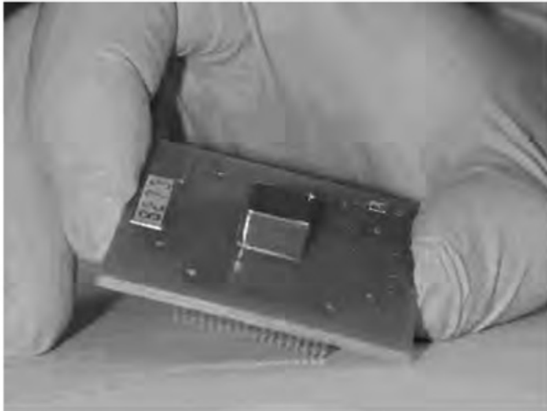
Fig. 18. 6 mm thick CZT array manufactured by eV-Products [photo from CEA-Saclay].
