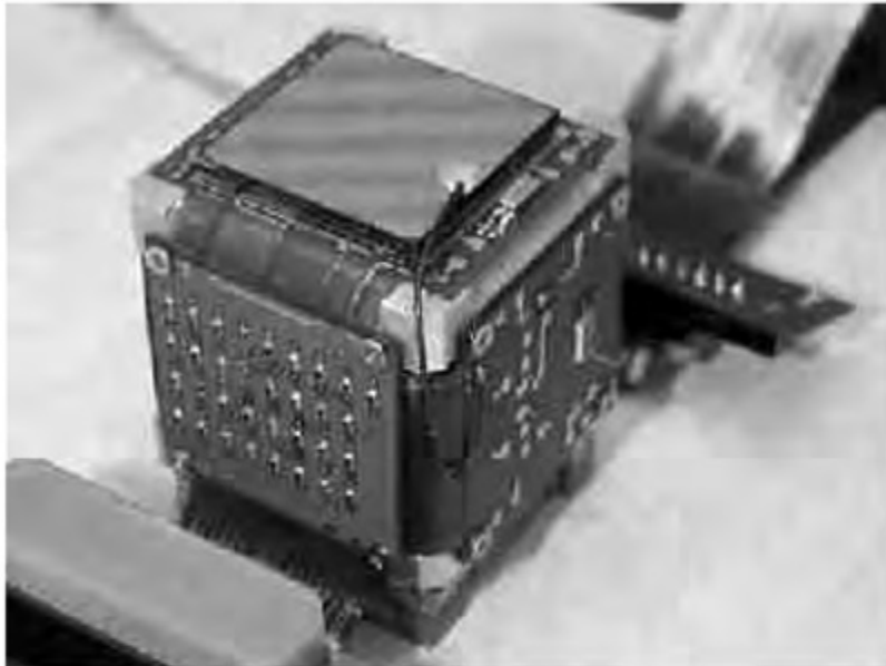
Fig. 14. Compact hybrid package CdZnTe/ASIC for the InFOCpS experiment. Gold coplanar contact on the cathode of the detector is visible on top with wire attached. The readout ASIC is underneath the detector [25].
