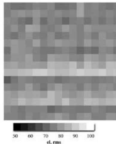
Fig. 4. Equivalent noise charge map for Caliste 256 SN2.
