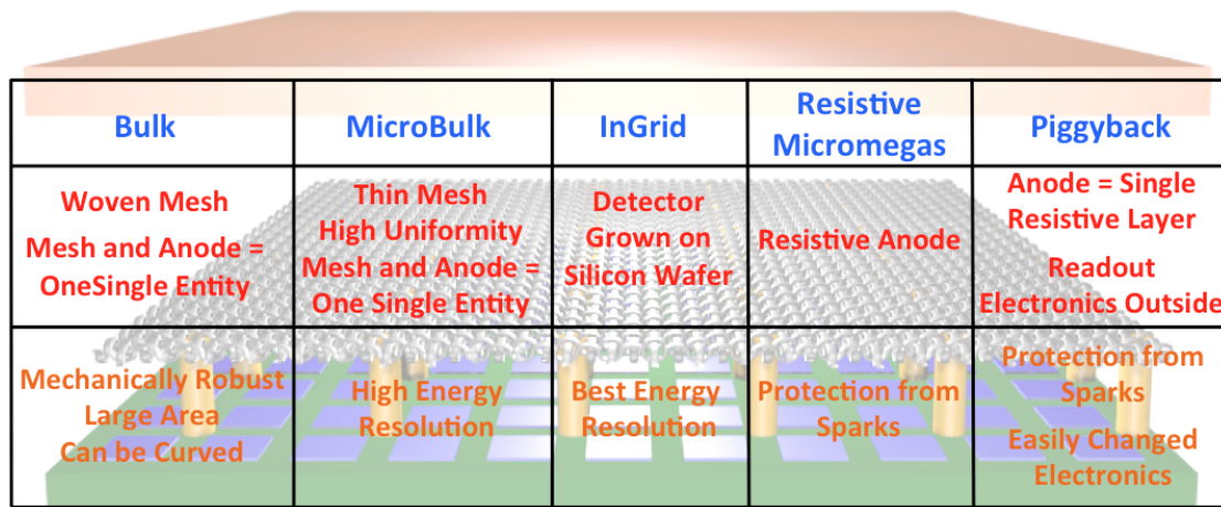
Figure 2.19: The Micromegas architecture family.
