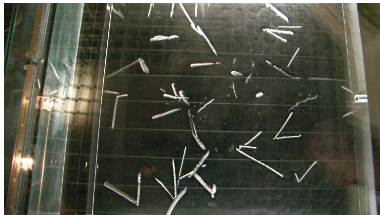
FIGURE II.1 – Saclay Wilson chamber showing the disintegration of ^{220}\text{Rn} .
