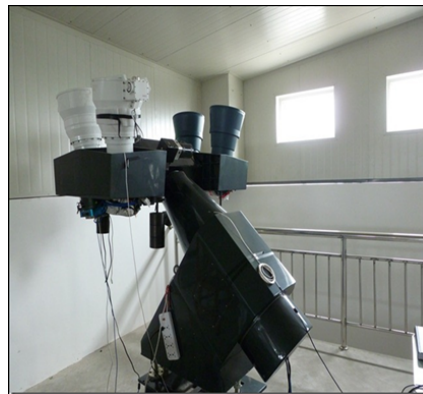
FIGURE 2.10 – Instrument Ground based Wide Angle Cameras (Crédits : NAOC).
