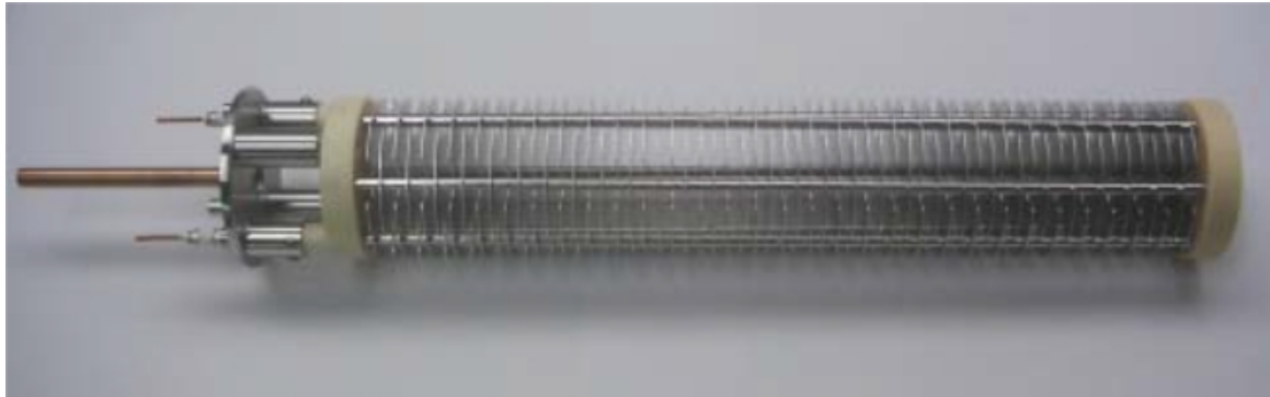
Figure 2.12 – The ionization chamber of an icBLM.
