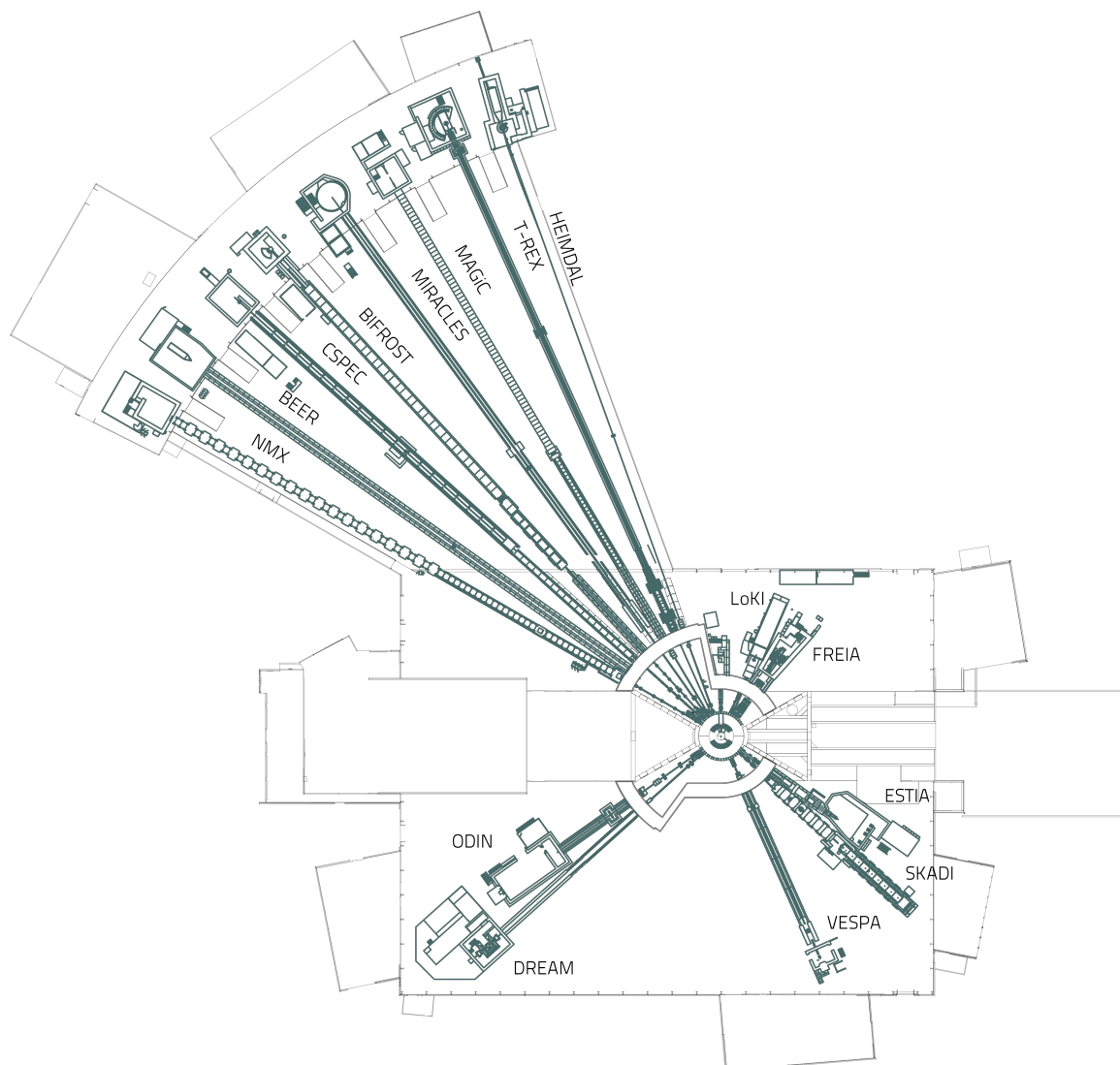
Figure 2.9 – Scheme of the 15 neutron instruments that will be available at the start of the user program.
