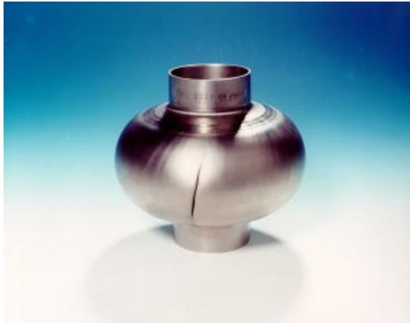
Fig.3 : The maximum deformation obtained for 1.3 GHz cavity hydroforming
