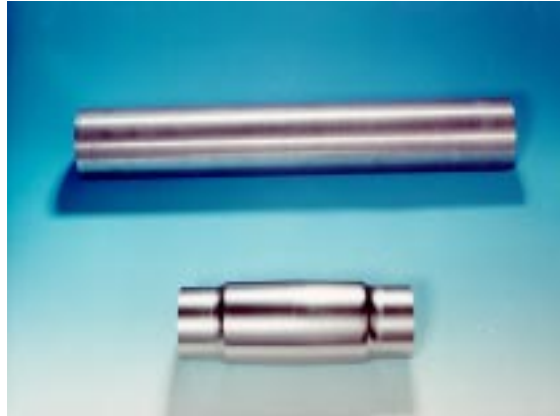
Figure 1 : Raw Nb tube and Nb tube prepared for 1-Cell hydroforming
