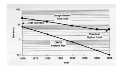
Figure 1: Sensor pixel size versus year, CMOS design rule versus year (after [FOSS97])
