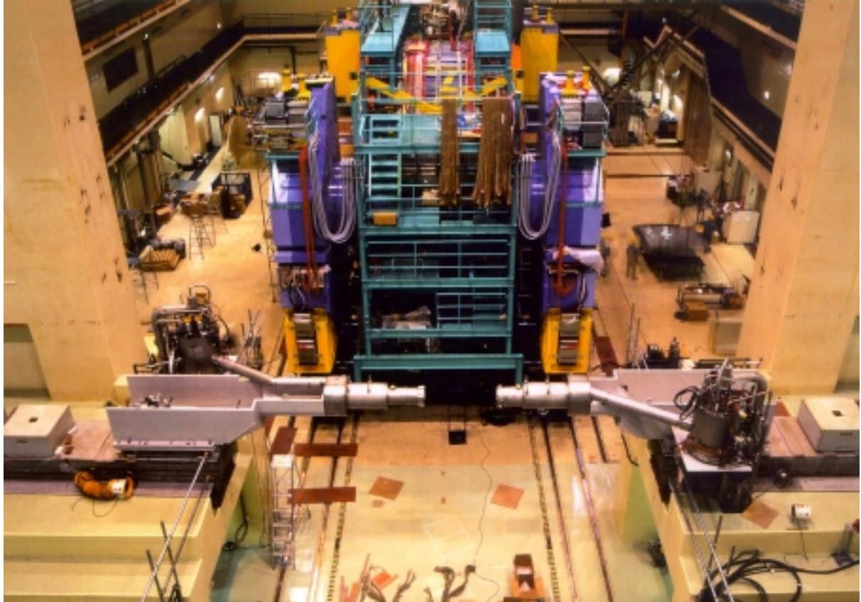
Figure 7. Implementation of the final focusing quadrupole magnets for the KEK-B factory. The magnets are shown in front of the BELLE detector, which has been railed back from its normal position.
