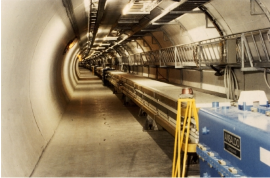
Figure 6. View of the conventional electromagnet ring of the LEP collider at CERN.
