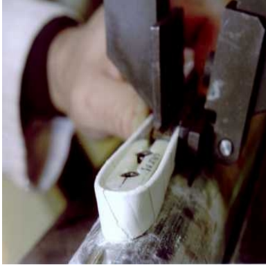
Fig. 6. Bending test on un-reacted Nb 3 Sn cable wrapped with innovative pre-impregnated fiber tape at CEA/Saclay.
