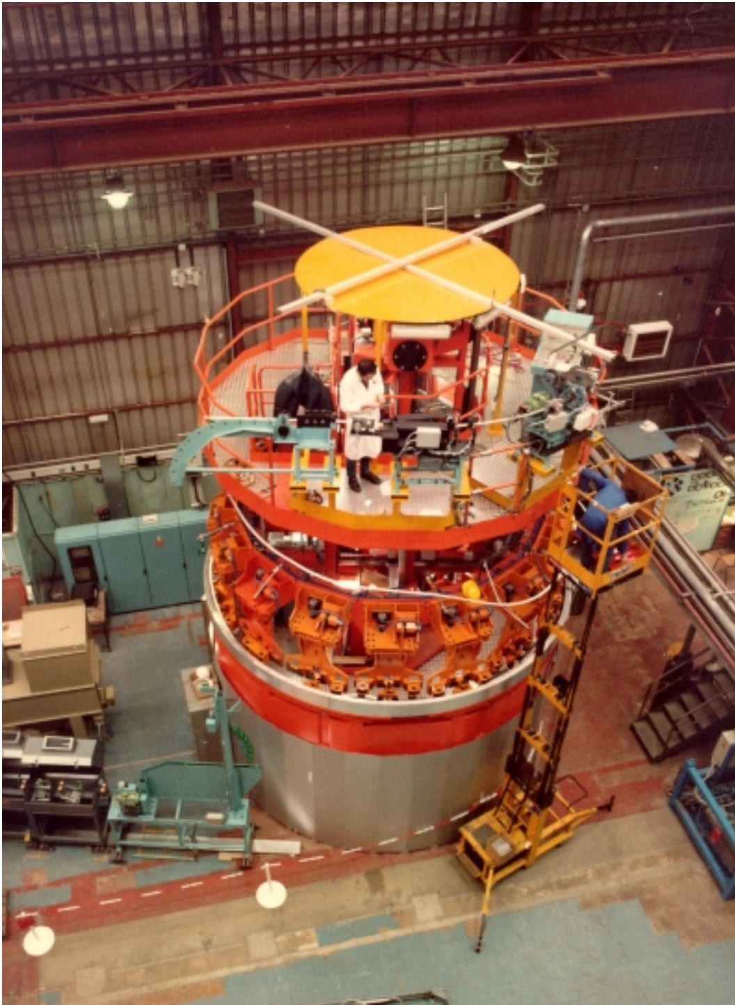
Winding of ALEPH Solenoid at CEA/Saclay.
