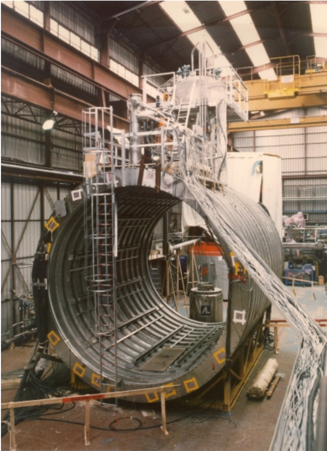
ALEPH Solenoid Undergoing Cold Tests at CEA/Saclay.
