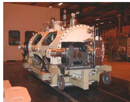
Figure 3 : Cryomodule in front of the CERN clean room
