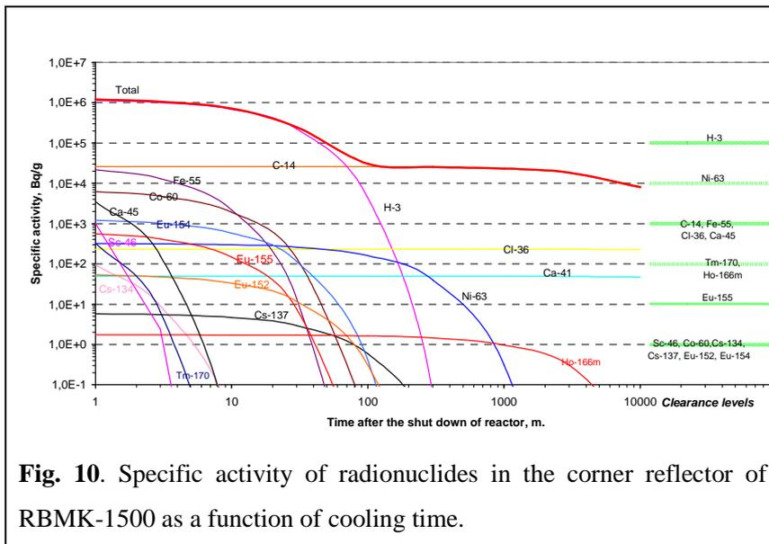
**Fig. 10.** Specific activity of radionuclides in the corner reflector of RBMK-1500 as a function of cooling time.
