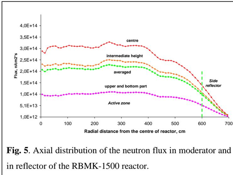
To evaluate how the neutron flux and its energy distribution in the moderator are sensible to the fuel burn-up and the presence of control rods, three models having the same basic geometry but a few important differences have been employed. Model I uses fresh fuel and has no control rods. The fresh fuel is replaced with the fuel of 10 MWd/kgU burn-up in model II (composition of
