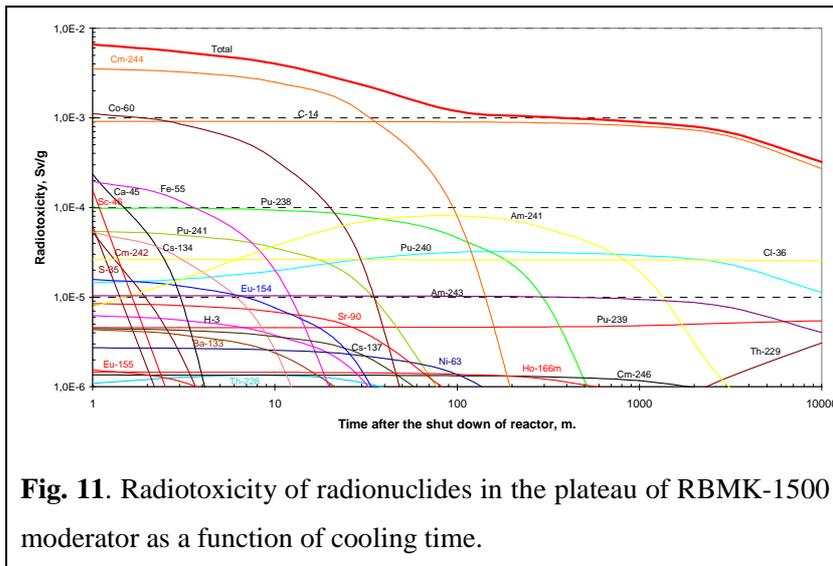
**Fig. 11.** Radiotoxicity of radionuclides in the plateau of RBMK-1500 moderator as a function of cooling time.
