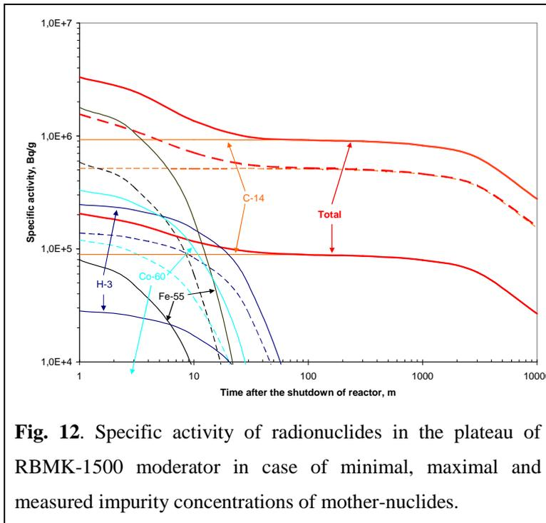
**Fig. 12.** Specific activity of radionuclides in the plateau of RBMK-1500 moderator in case of minimal, maximal and measured impurity concentrations of mother-nuclides.
