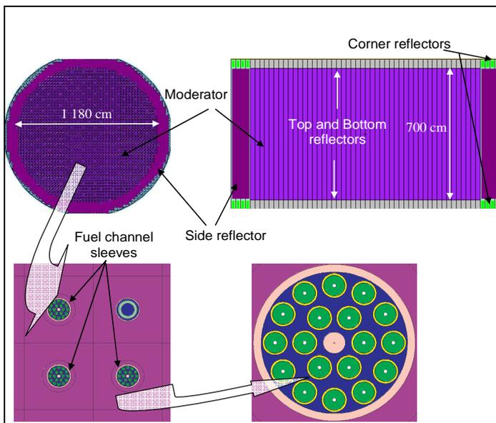
**Fig. 2.** The MCNPX model of RBMK-1500 reactor with horizontal and vertical sections (top), 4 lattice elements containing (bottom): moderator prisms, fuel channel sleeves, 3 fuel channels with 18 fuel rods, and a control rod. A single fuel channel is also presented separately.
