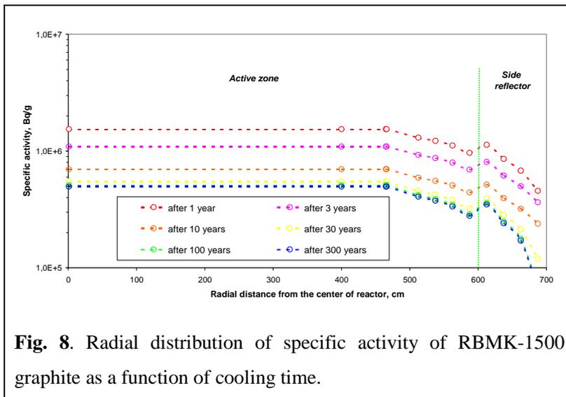
**Fig. 8.** Radial distribution of specific activity of RBMK-1500 graphite as a function of cooling time.
