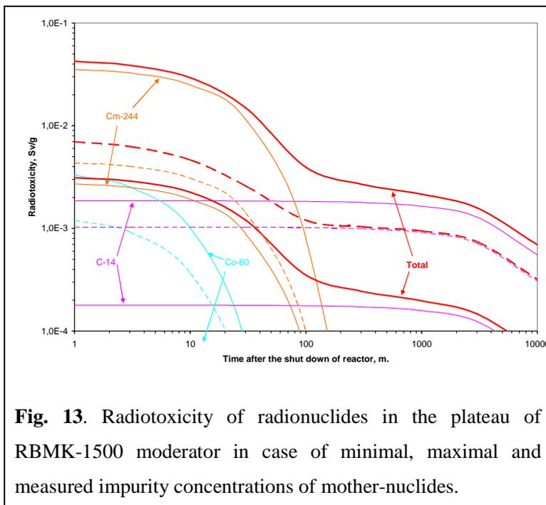
**Fig. 13.** Radiotoxicity of radionuclides in the plateau of RBMK-1500 moderator in case of minimal, maximal and measured impurity concentrations of mother-nuclides.
