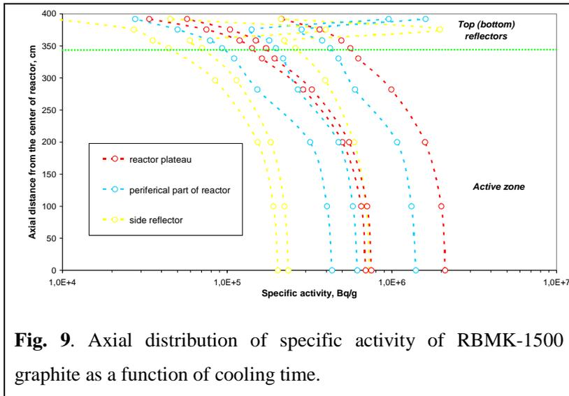
**Fig. 9.** Axial distribution of specific activity of RBMK-1500 graphite as a function of cooling time.
