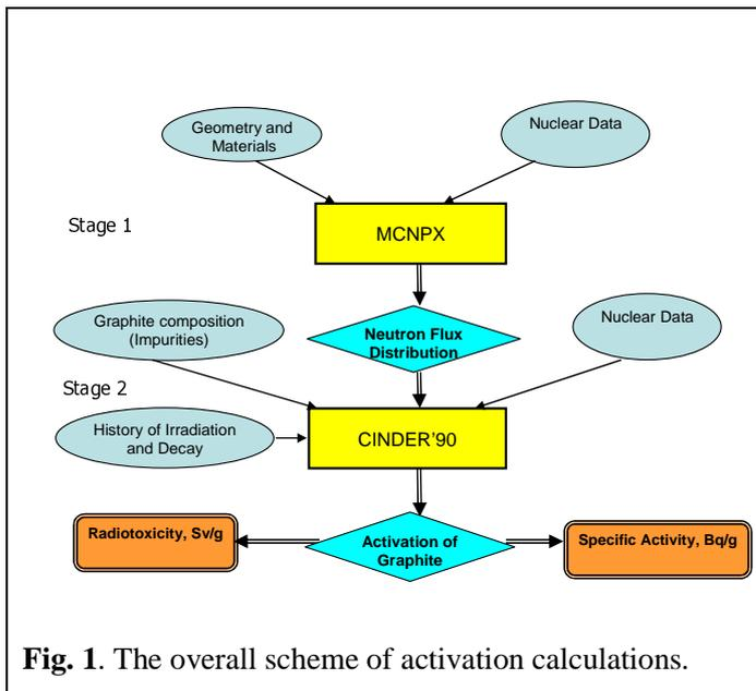
The activation code also needs the chemical composition and impurities of graphite. The specimen of the fresh RBMK-1500 graphite taken from the fuel channel sleeve has been analyzed in Saclay Research Centre of French Atomic Energy Commission (CEA) by 2 independent methods: gamma spectroscopy based on activation by neutrons and glow discharge mass spectroscopy (GDMS).
