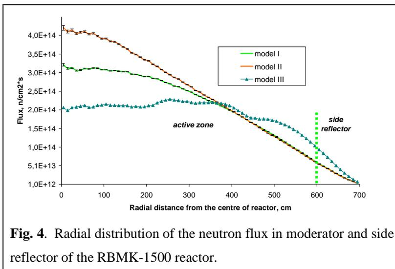
to 800 °K and 600 °K, which are close to the realistic operational temperatures. The density of water in model is 0.5 g/cm<sup>3</sup> and of graphite – 1.675 g/cm<sup>3</sup>. The neutron flux and its energy spectrum are calculated in each of the above mentioned graphite constructions. Fig. 3
