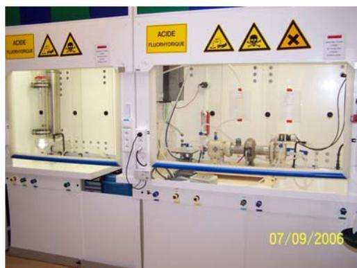
Figure 1: Electro-polishing set-up at CEA Saclay.
