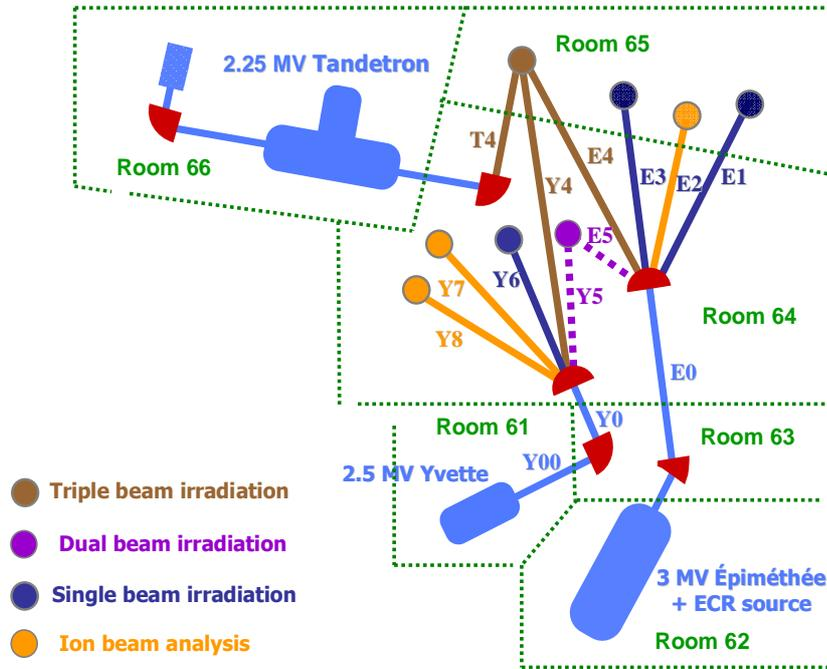
**Figure 2: General layout of the Orsay's dual beam facility coupled with a 200 kV TEM.**
