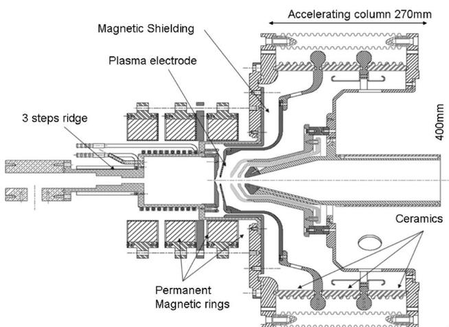
FIG. 2. The five-electrode extraction system.
