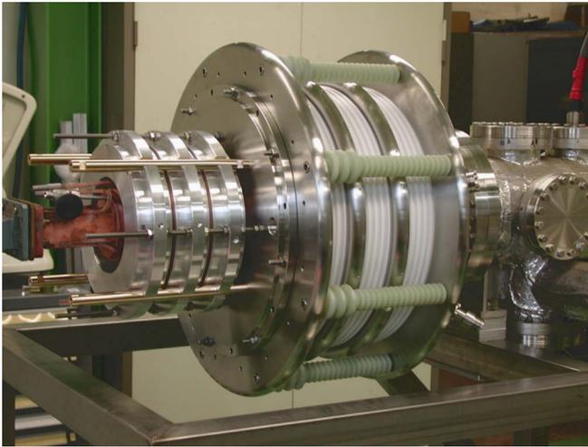
FIG. 1. (Color online) Permanent magnet source adapted on the modified SILHI accelerating column.
