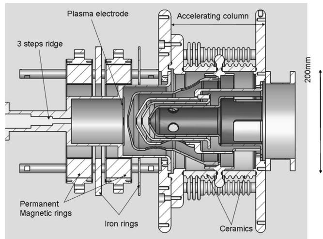
FIG. 3. Compact accelerator column on BETSI.
