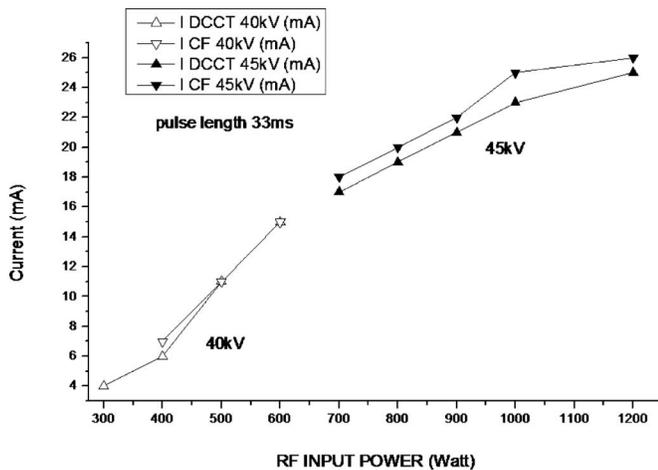
FIG. 4. Extracted and drain current vs rf input power for two high voltage potentials with pulse length of 33 ms.
