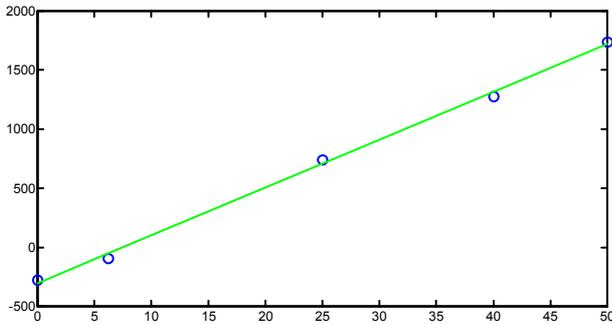
Figure 4: 3D frequency shift (kHz) vs. tuner position even part  $h_{QQ0}$  (mm). 0 kHz reference: 2D simulation.
