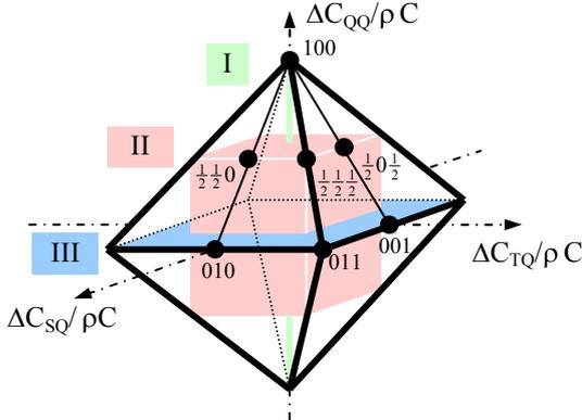
Figure 6: Inter-vane capacitance errors envelope.
