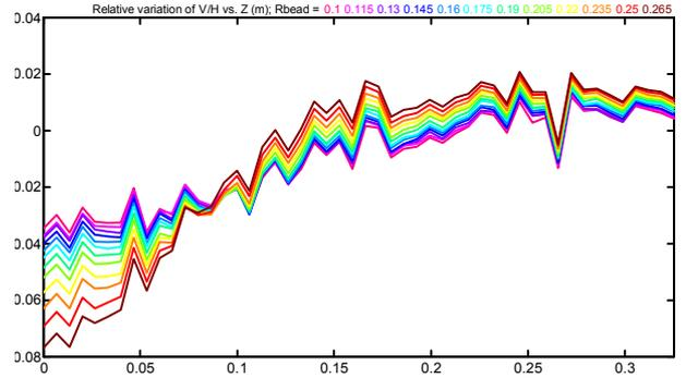
Figure 5:  $[\kappa(z) - \kappa^0]/\kappa^0$  vs.  $z$  for various bead position radii (color). Position of tuner located at  $z = 0$  is  $+50$  mm.
