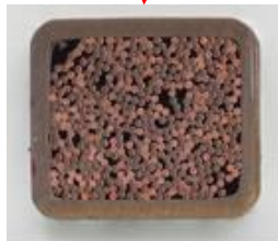
Cross section of conductor (NbTi/Cu)
