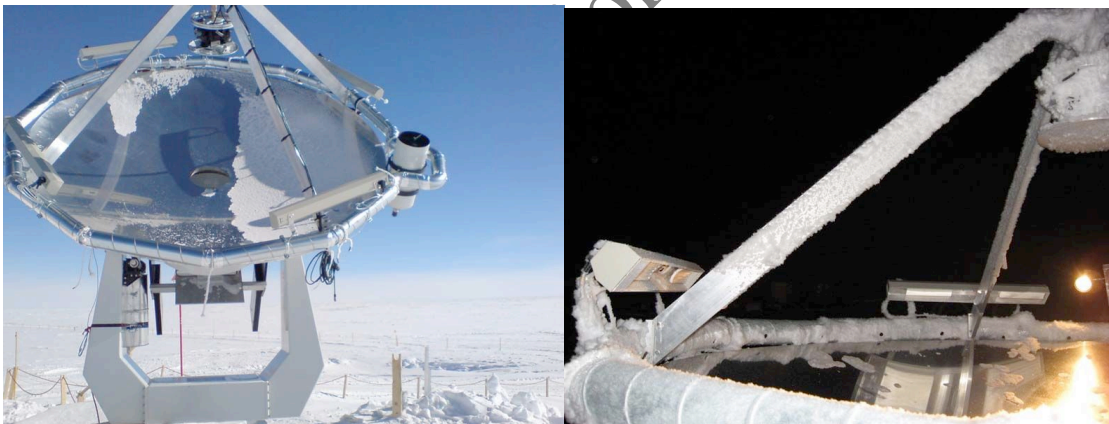
Figure 11.3: Left: The Italian 2.6m telescope Cochise equipped with infrared heaters, 24 holes to blow dry air and a heating system on the mirror. An efficient combination is a small warm up of the telescope to make the surface slippery in addition to blowers to flush the snow. Right: The infrared heaters remove the snow from the M2 support. This unprotected mirror accumulates frost toward the bottom. The M1 mirror in horizontal position is nearly clean. By tilting it, the snow would fall down.
