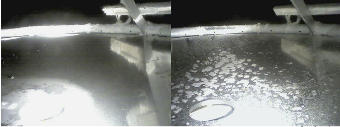
Figure 11.4: Left: On this web-cam photo, the mirror is heated 5°C above ambient. The snow is pushed toward the centre of the mirror by both gravity and the blower. Right: Without a cleaning anti-frost system, the mirror is rapidly covered with frost and snow.
