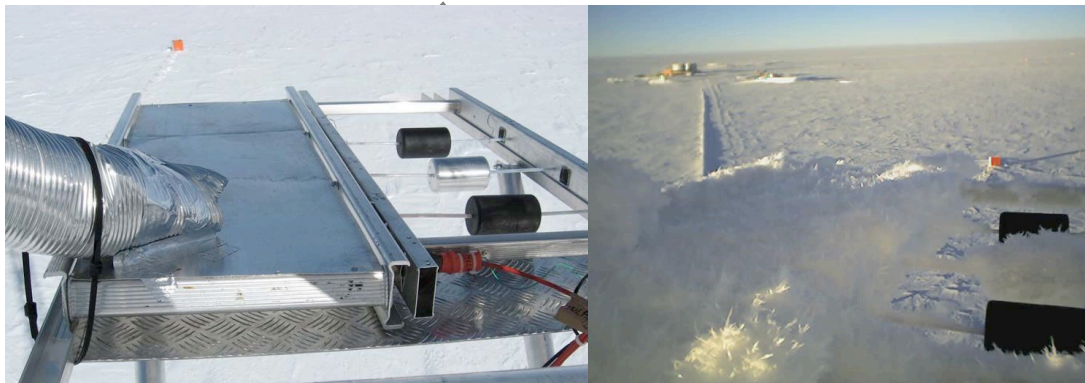
Figure 11.1: Left: At 30m a shiny aluminium surface is blown with dry air from the ground level, near the 3 heated frost cells. Right: At 30m up to 6°C above ambient are sometimes needed to keep the cells clear of frost. The blower is not active on this photo. The crystals are typical frost built-up.
