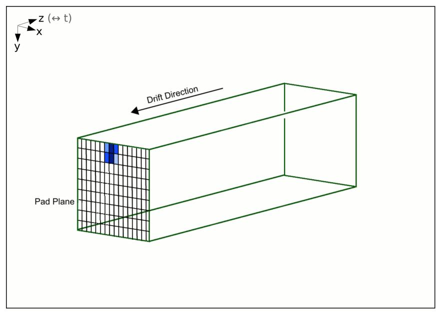
Integration over time of the signal on the pad plane
