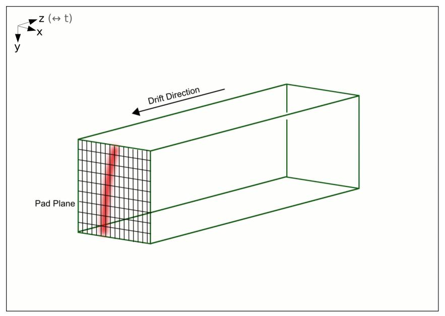
Now the signal on the single pads: since track is inclined, some parts arrive earlier
