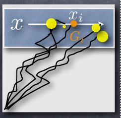
Again we assume that the charged particle passed through the TPC at x=0 parallel with the readout plane and perpendicular to the pad rows.
