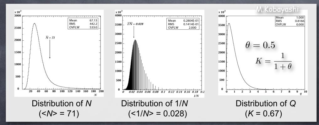
In the case of Snyder's model, gain fluctuation is exponential and K=1 (theta=0) and the Neff is reduced by a factor of 2 by it. In the case of Legler's model, theta>0 and the reduction is less sever. If we assume theta=0.5, for instance, we have a factor of 1.5 reduction:  $((C)^2)$
