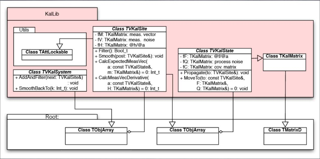
A TVKalSite carries predicted, filtered, and smoothed TVKalState's Application-specific functions are pure virtual and to be implemented in a derived class
