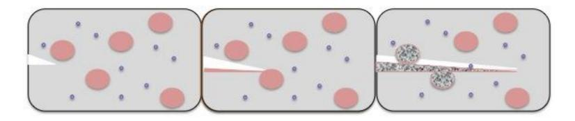
Depiction of crack propagation through microcapsule-imbedded material. Monomer microcapsules are represented by pink circles and catalyst is shown by purple dots.
