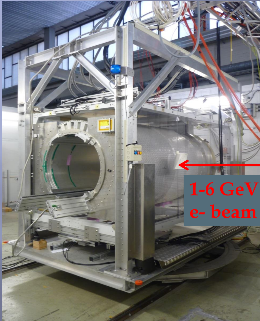
The movable stage and the 1T magnet.
