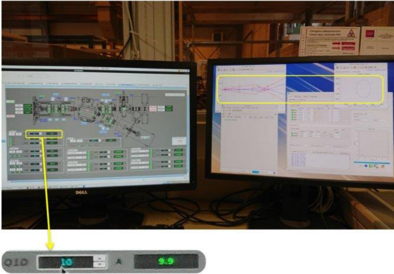
Views of IPHI's control room. QD1 is set by operator to 10A, new VA simulation is launched and new output displays are synchronized.
