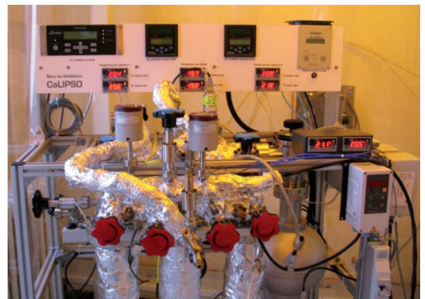
Full features TMBi purification bench for the CaLIPSO project.
