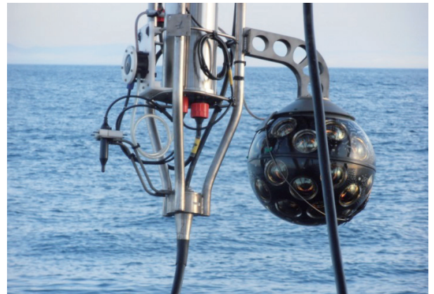
Picture of the digital optical module prototype during deployment in April 2013. For this occasion, the prototype was connected to the ANTARES instrumental line.
