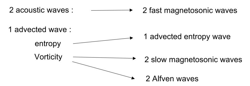
Vorticity and entropy decouple : vorticity can propagate!
