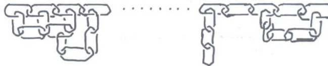
Fig. 5. Complex chain of dislocation loops.
