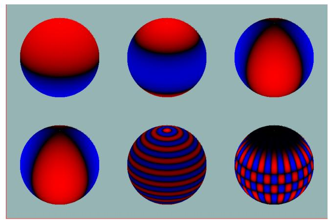
•Behave like spherical harmonics:  $P_l^m(\cos \theta) \cos(m \phi - \omega t)$ • $k_h = 2 \pi / \lambda_h = [l(l+1)]^{1/2}/r$
