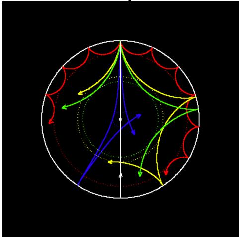
$$k_r = \left[\frac{\omega^2}{c^2} - \frac{l(l+1)}{r^2}\right]^{1/2} \qquad \text{Turning point: } \frac{c(r_t)}{r_t} = \frac{\omega}{\sqrt{l(l+1)}}$$
