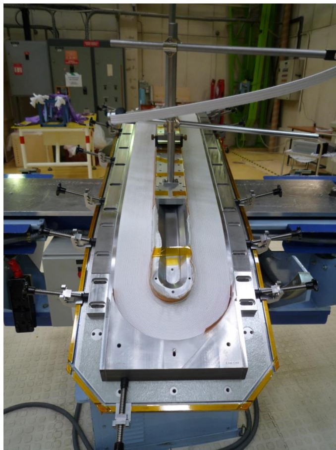
Fig. 7.7.1 – Winding test of full-size copper coil CC3401 (first layer complete).
