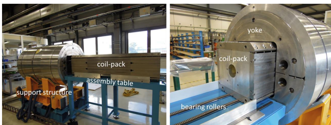
Fig. 6.4.21 – Assembly table, insertion of the coil-pack.
