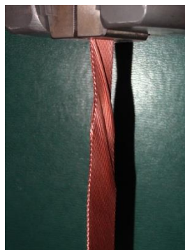
Fig. 7.5.3 – Traction test on FRESCA2 cable.
