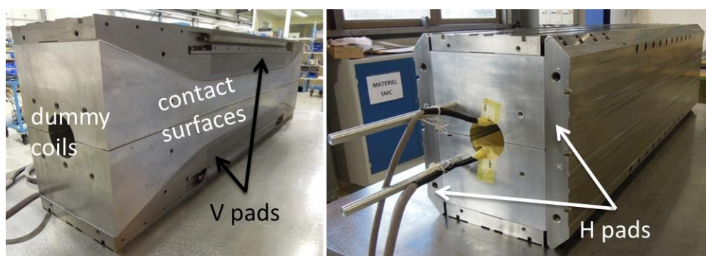
Fig. 6.4.10 – Coil-pack with dummy-coils.
