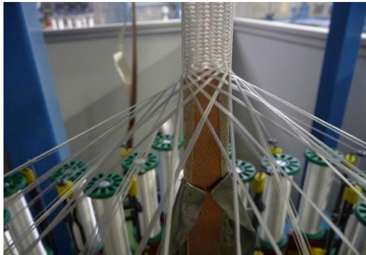
Fig. 3.3.1 – S-grade fibre-glass braided around a cable.
