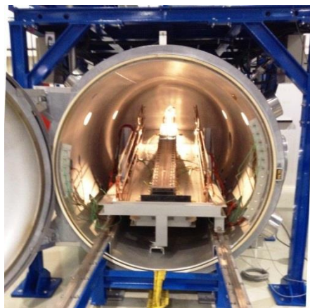
Fig. 6.3.1 – Vacuum chamber used for impregnation.
