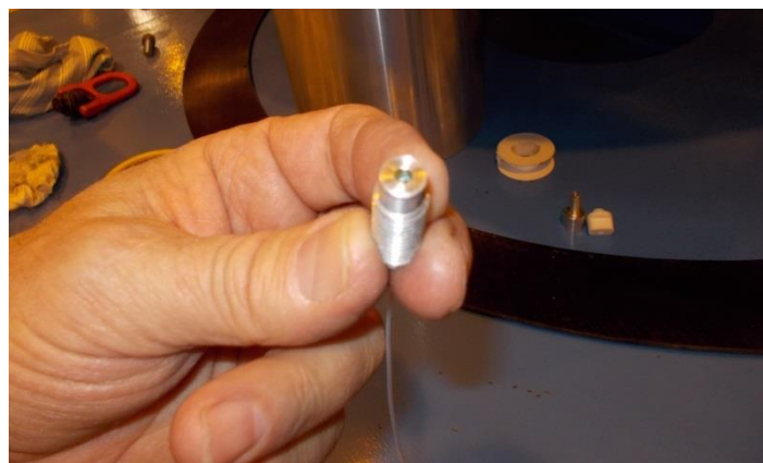
Fig. 7.8.5 – Temperature sensor.
