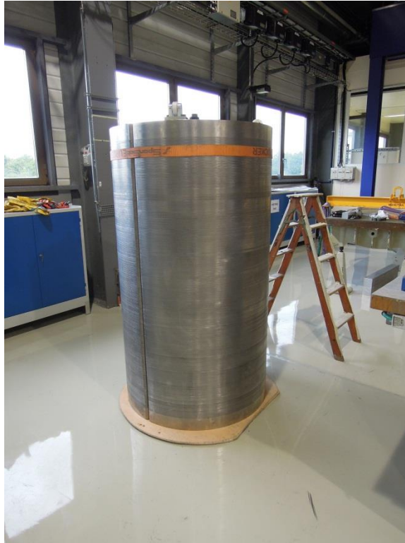
Fig. 6.4.13 – Structure assembly: the halve yokes into contact.
