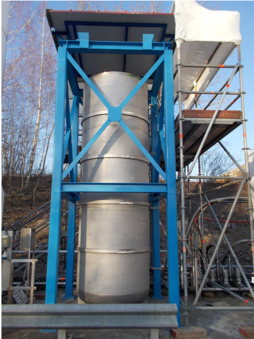
Fig. 7.8.9 – Vessel of Ø1.2m x 4m for the cool-down test outside of SM18.
