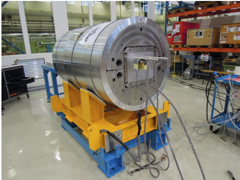
Fig. 6.4.22 – Coil-pack inserted into the yoke.
