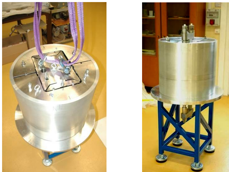
Fig. 5.1: SMC structure on its support, with dummy coil pack inside
