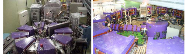
Figure 1: (a) The 500 keV (left) and (b) 150 MeV (right) proton scaling FFAGs built at the KEK laboratory in Japan
